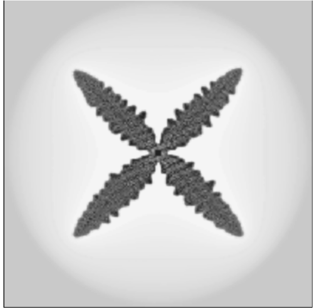
FIG. 5. Same as Fig. 2, but a conservative Langevin noise term is added to the equations of motion: sidebranches appear.
